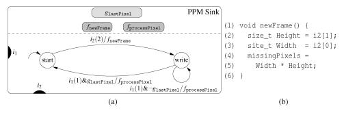
Fig. 3. (a) Depiction of the *PPM Sink* actor from Figure 1 consisting of two input ports  $i_1$  and  $i_2$ , a set of *actions* and *guards* and the state machine that determines its communication behavior. The transitions of the state machine are annotated with *activation pattern/action* pairs. (b) shows the source code of the action  $f_{newFrame}$ .
