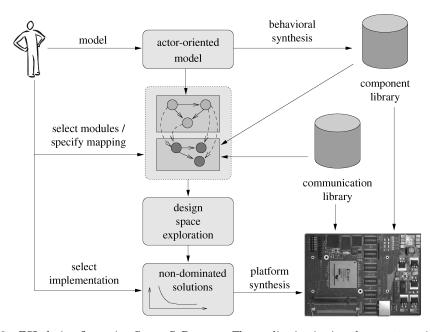
Fig. 2. ESL design flow using SYSTEMCODESIGNER: The application is given by an actor-oriented model described in SystemC. Behavioral synthesis is used to create *architecture templates*. Design space exploration using *multi-objective evolutionary algorithms* automatically searches for the best architecture candidates. The entire SoC is implemented automatically for FPGA-based platforms.
