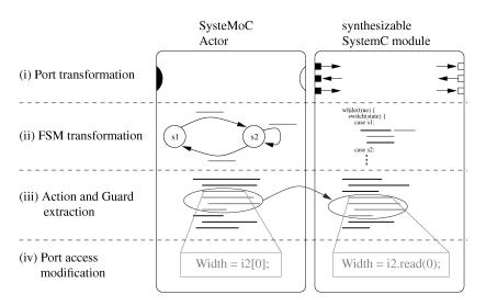
Fig. 4. Transformation steps of a SysteMoC actor to a synthesizable SystemC module.
