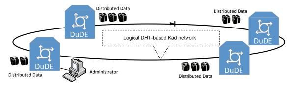
Fig. 3. Kad-based DHT ring connecting DuDE nodes for distributed statistics computing and distributed data storage.
