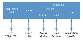
Fig. 1. General data storage interface for clouds [11]
