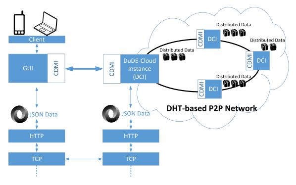
Fig. 4. DuDE-Cloud concept combining the P2P network with CDMI.
