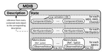
Fig. 3. Schematic illustration of selected (partial) states of the device state (speech bubble contain example values)
