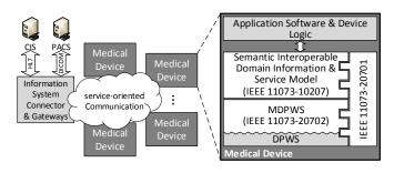
Fig. 1. Schematic overview of the device communication and the new IEEE 11073 Standards
