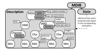
Fig. 2. Schematic overview of device capability modeling (example containment tree; speech bubbles contain example content)
