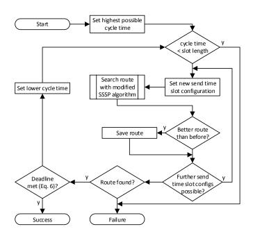
Fig. 4. Flowchart of the main part of the routing and scheduling algorithm.
