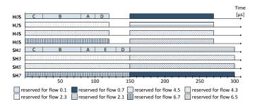
Fig. 5. Link Schedule for the presented test case. Reservation consists of: A: Actual transmission time slot B: Safety margin for variable software delay C: Safety margin for synchronization inaccuracy (early clock) D: Safety margin for synchronization inaccuracy (late clock) E: Safety margin for variable switch delay.
