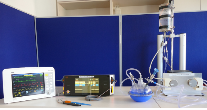
Fig. 3: Demonstrator (f.r.t.l.): research prototype of a smart surgical pump (implementing the Rule Execution Engine ), knee phantom, HF surgical device and patient monitor.
