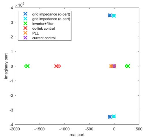
Fig. 7: root locus for small-signal behaviour of VOC with increasing dc-link capacitance
