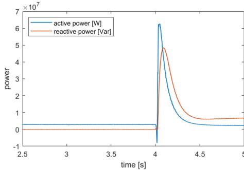
Fig. 6: output power of converter
