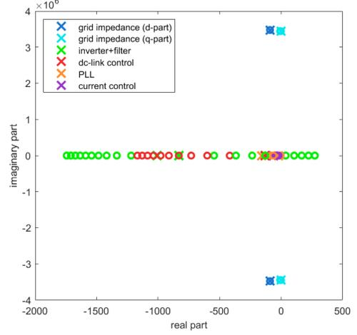
Fig. 3: whole plot of root locus for small-signal behaviour of VOC with increasing droop gain
