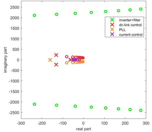
Fig. 4: zoom in of root locus for small-signal behaviour of VOC with increasing droop gain
