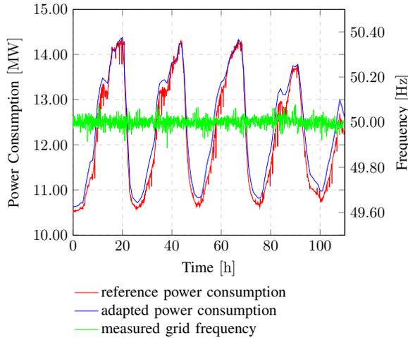
Fig. 6. Power consumption comparison between the reference data center model and main frequency adapting data center with a measured main frequency data
