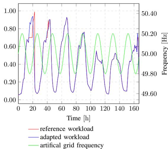
Fig. 5. Workload comparison between the reference data center model and main frequency adapting data center with an artificial sine wave frequency
