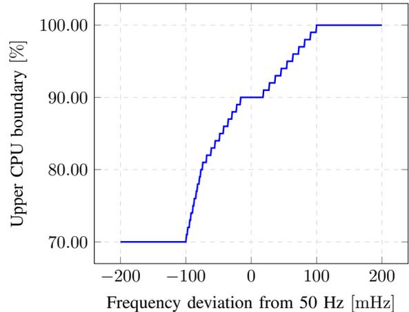
Fig. 1. Upper CPU frequency boundary dependent on the main frequency deviation
