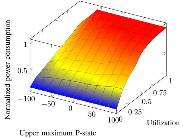
Fig. 3. Normalized power consumption of an Intel Core i7 9700 for different loads and varying allowed maximum P-state
