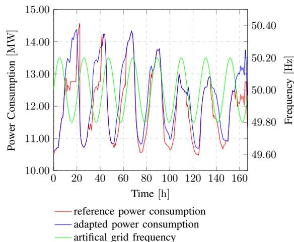
Fig. 4. Power consumption comparison between the reference data center model and main frequency adapting data center with an artificial sine wave frequency
