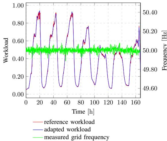
Fig. 7. Workload comparison between the reference data center model and main frequency adapting data center with a measured main frequency data
