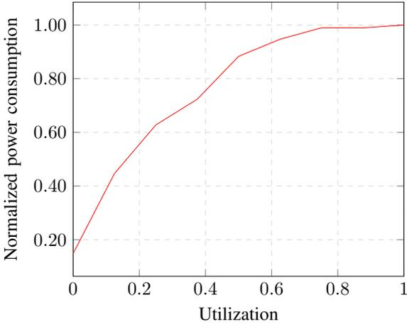
Fig. 2. Normalized power consumption of an Intel Core i7 9700 dependent on the utilization
