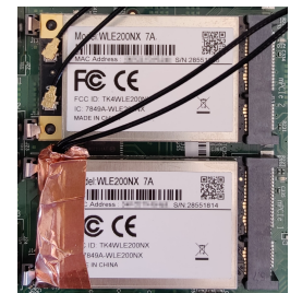
Fig. 4: Pigtail copper shielding
