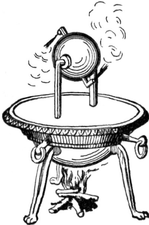
Aeolipile (Heron's ball), Heron von Alexandria, Antike
